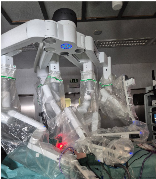
Figure 5. Da Vinci docked, 3 arms: 1. Prograsp fenestrated forceps; 2. 30° endoscope; 3. Ultracision harmonic scalpel.
